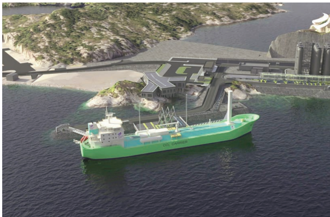
The Northern Lights JV has ordered two 7,500m 3 -capacity dedicated CO 2 carriers from Dalian Shipbuilding Industry Co., Ltd. (DSIC) which will be used to transport liquid CO 2 from European emitters to Northern Lights' Øygarden receiving terminal in Norway
