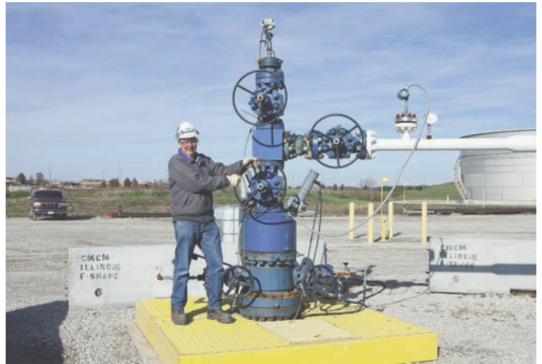
Rob Finley, principal investigator on the Illinois Basin-Decatur Project, turns the main valve to start injection of CO2 into the Mt. Simon saline reservoir. | Daniel Byers/ Illinois State Geological Survey
