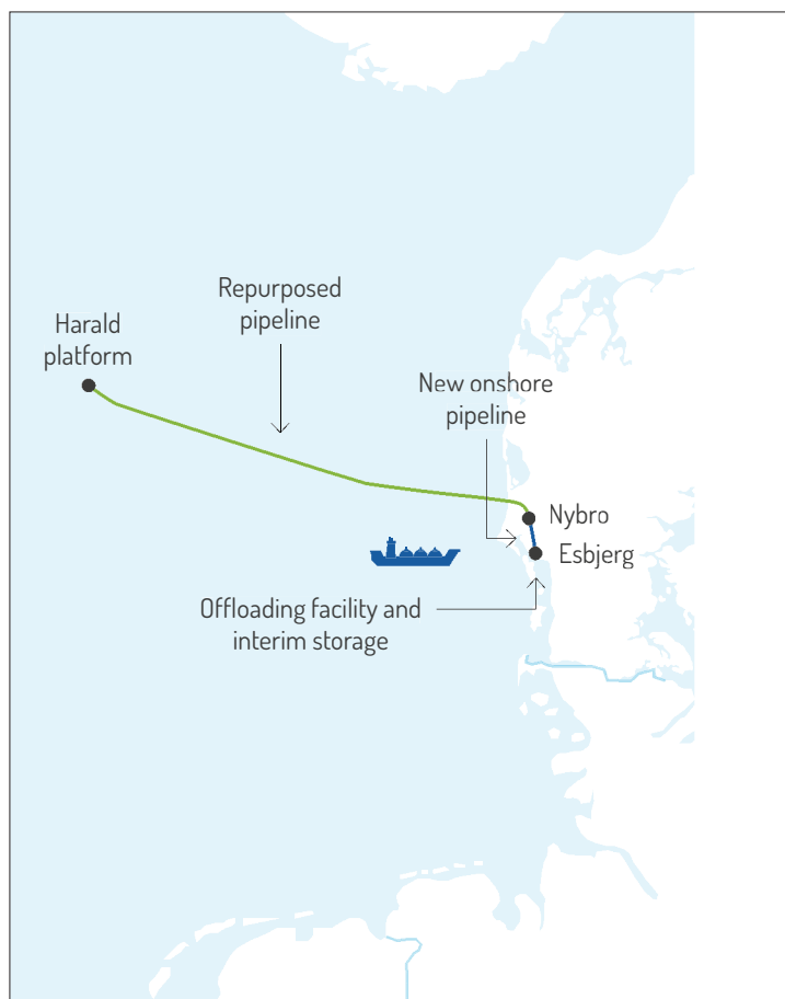
Both a repurposed pipeline and a shipping solution are being explored to transport CO 2 to the Harald platform 250km offshore Denmark
