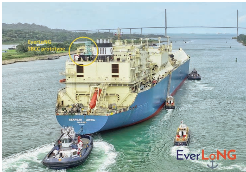
LNG carrier chartered by TotalEnergies containing the CO 2 capture unit (Image courtesy Seapeak Arwa)
