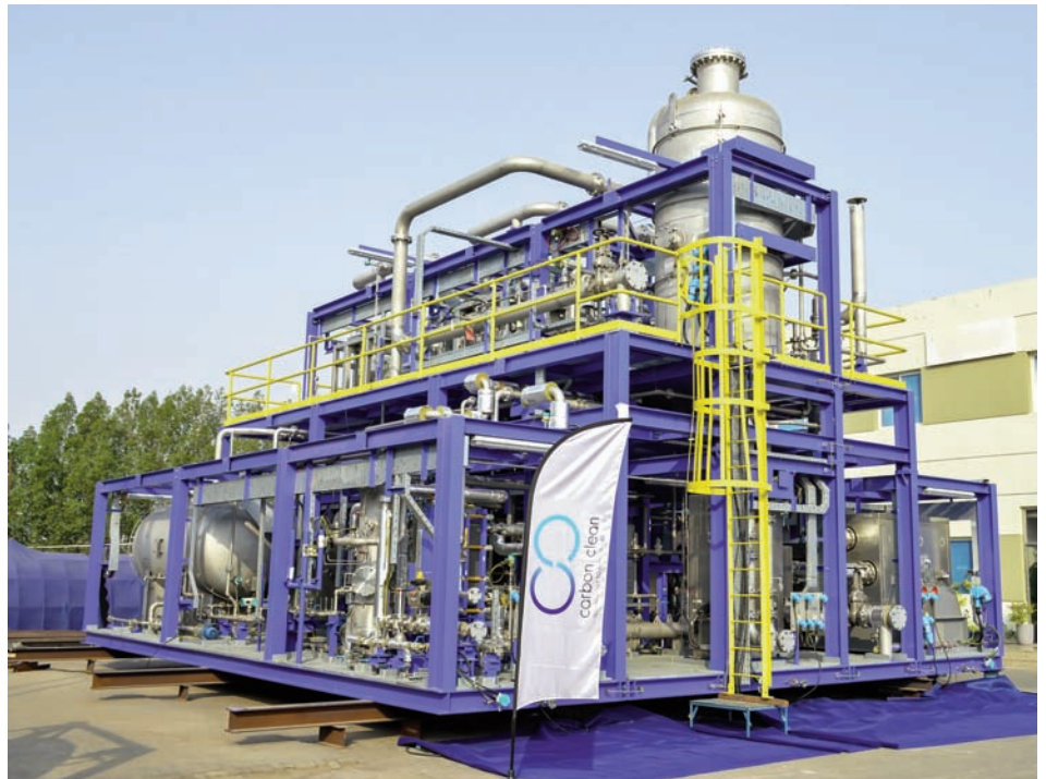
The modular CycloneCC carbon capture technology is well suited to offshore maritime use due to its small footprint and enhanced performance under vessel motions
