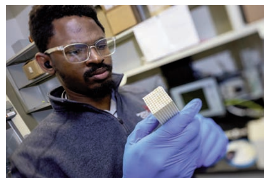
UC doctoral student James Akinjide holds up a honeycombed block covered in an adsorbent that captures carbon from air. Photo/Andrew Higley/UC Marketing + Brand
