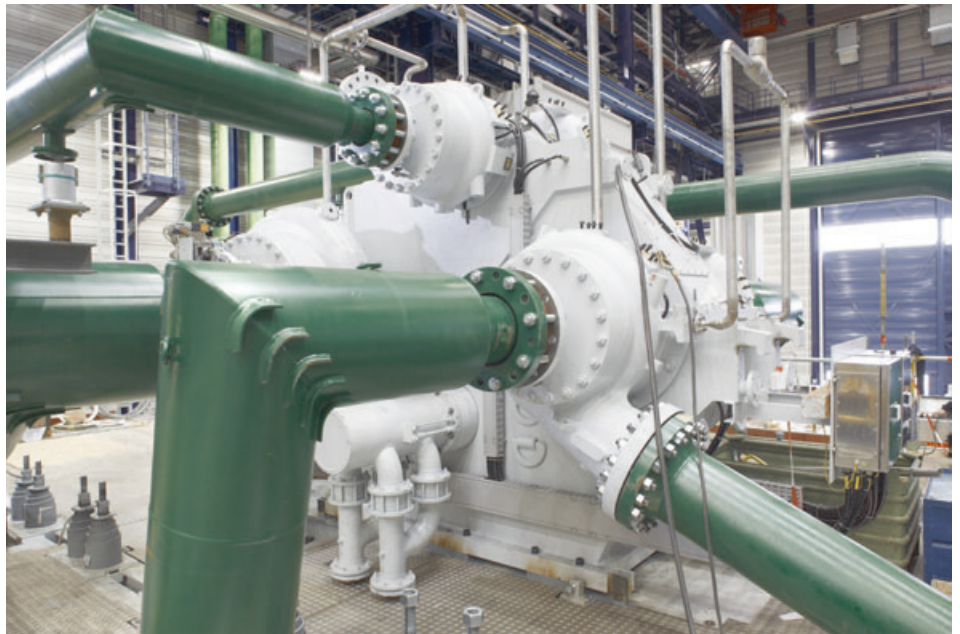
Siemens delivered compressors with a volume flow rate of 83,000 m 3 /h for a coal liquefaction plant in Yinchuan, Ningxia Province, in the northwestern part of China for Shenhua Ningxia
