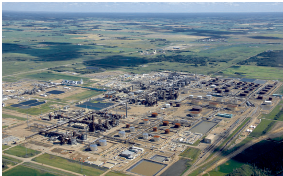
Aerial view of Shell Scotford located 40 kilometres northeast of Edmonton, Alberta, Canada. Shell Scotford includes both a refinery, chemicals plant and oil sands upgrading facilities capable of producing 255,000 barrels per day of synthetic crude. Quest will capture and store more than one million tonnes of CO 2 per year from the Scotford Upgrader beginning in 2015 – which represents up to 35% of the direct emissions from the Upgrader (Image ©Shell)
