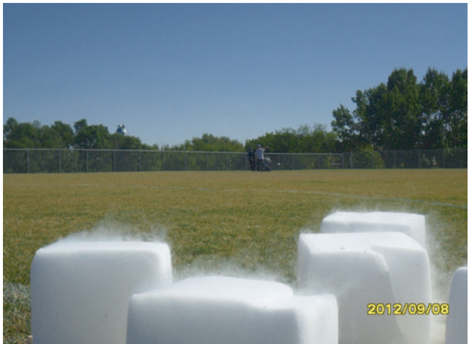
To field test the system, researchers placed six, 23-kilogram blocks of dry ice on a raised wooden platform in a soccer field, so that all sides of the dry ice could release CO 2 to the atmosphere
