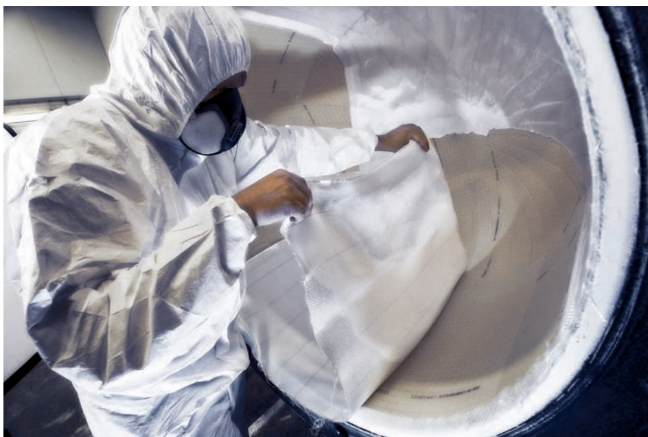
Composite moulding at Biobe AS. Composites or GRP have much better mechanical and temperature performances than most thermoplastics and can be used in very demanding products (Image: Biobe AS)
