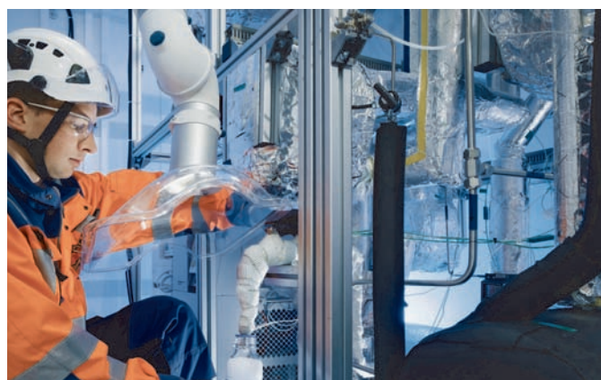
VTT's mobile synthesis unit MOBSU for bench-scale process development. (Photo by COMSYN-project)
