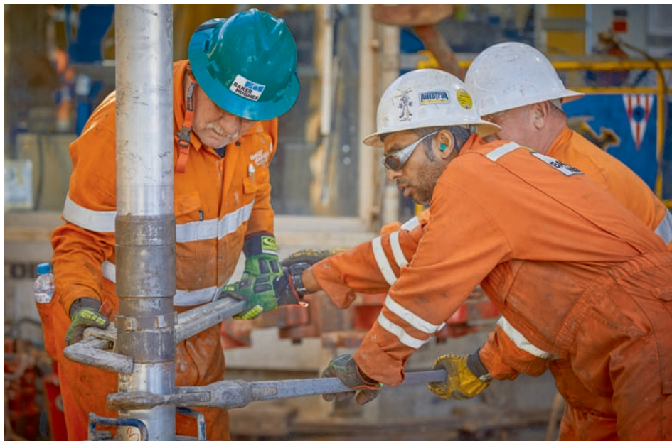
Extracting core rods at the Pelican site. The core samples will be analysed to detail their physical and chemical properties and confirm the site's suitability for CO 2 storage
