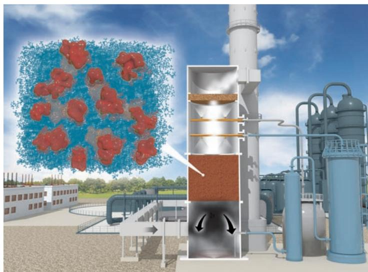
*The formation of clusters can degrade solvent performance in post-combustion CO<sub>2</sub> capture systems*
