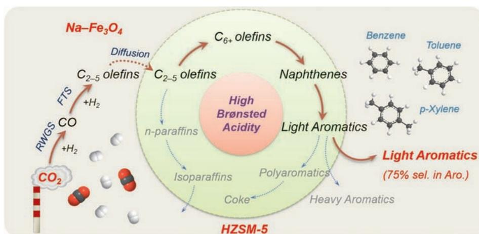
*Precisely regulating Brønsted acid sites to promote the synthesis of light aromatics via CO<sub>2</sub> hydrogenation (Image by WEI Jian and YAO Ruwei)*
