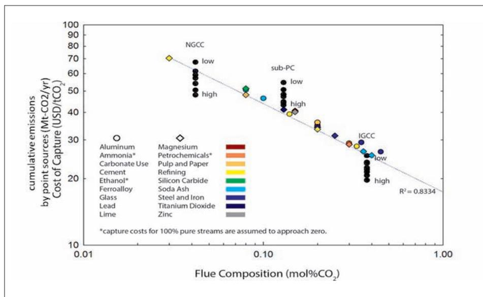
Figure 2 - Prediction of capture costs from a range of industrial sources (coloured symbols), and power generation (black circles) for low and high flow rates (Psarras et al., 2017)
