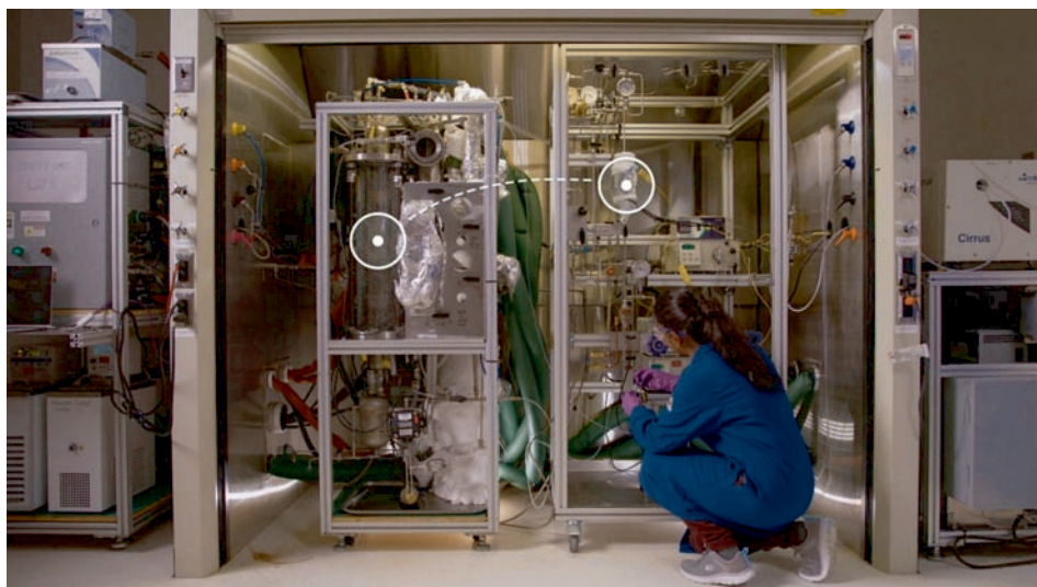
Taking up only as much space as a walk-in closet, a new carbon capture and conversion system is simple and efficient at removing carbon dioxide from gas that's rich with carbon dioxide. On the left of this walk-in fume hood, "smoke" moves through a cylindrical container where it makes contact with a carbon-capturing solvent. That solvent chemically binds to carbon dioxide and, on the right, is converted to methanol. (Photo by Eric Francavilla | Pacific Northwest National Laboratory)
