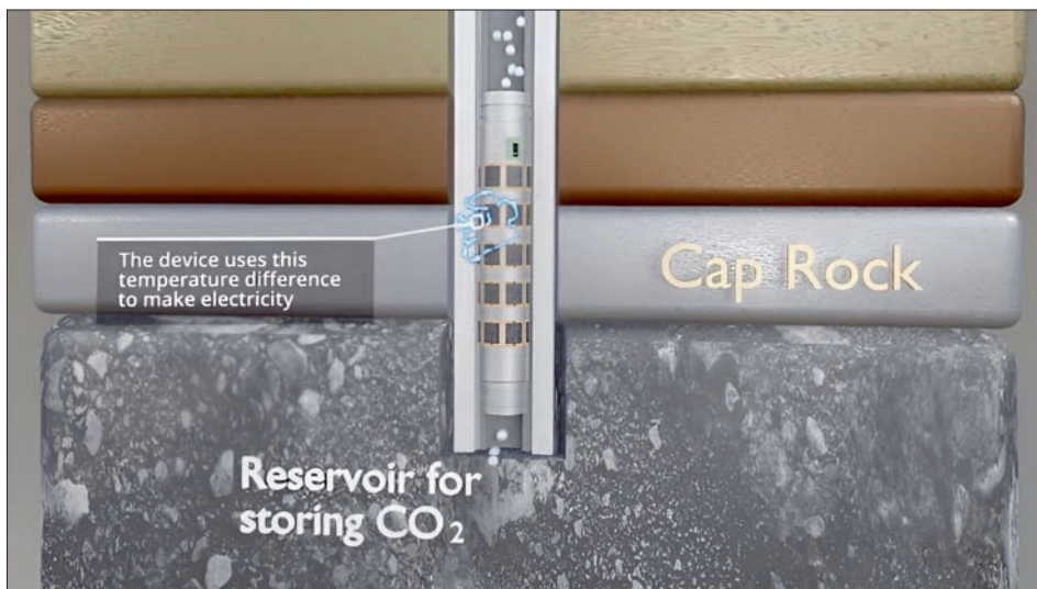
How Sandia National Laboratories' device could produce electricity at a carbon dioxide storage reservoir
