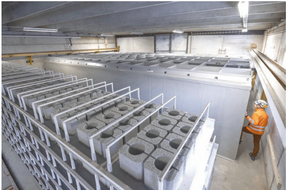
Carbonaide's first pilot plant in Hollola Finland where the CO 2 mineralised product is being made (Image: Carbonaide, photo by Vesa Kippola)
