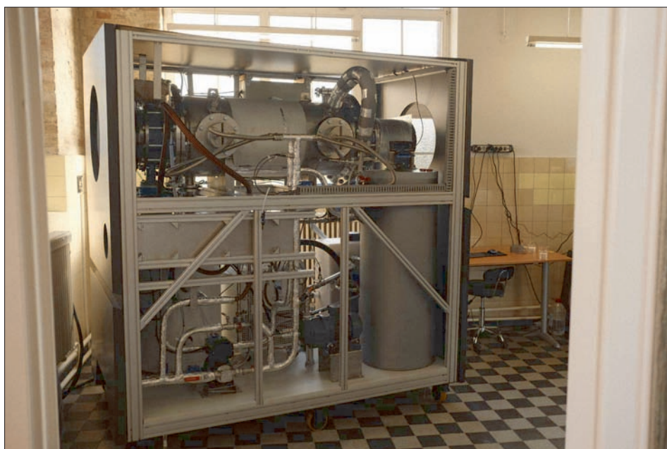
NeoCarbon technology reuses the heat that cooling systems normally evacuate, so minimal additional energy is used to capture CO 2 from the air. It can be retrofitted to many waste heat stream types and is fully scalable
