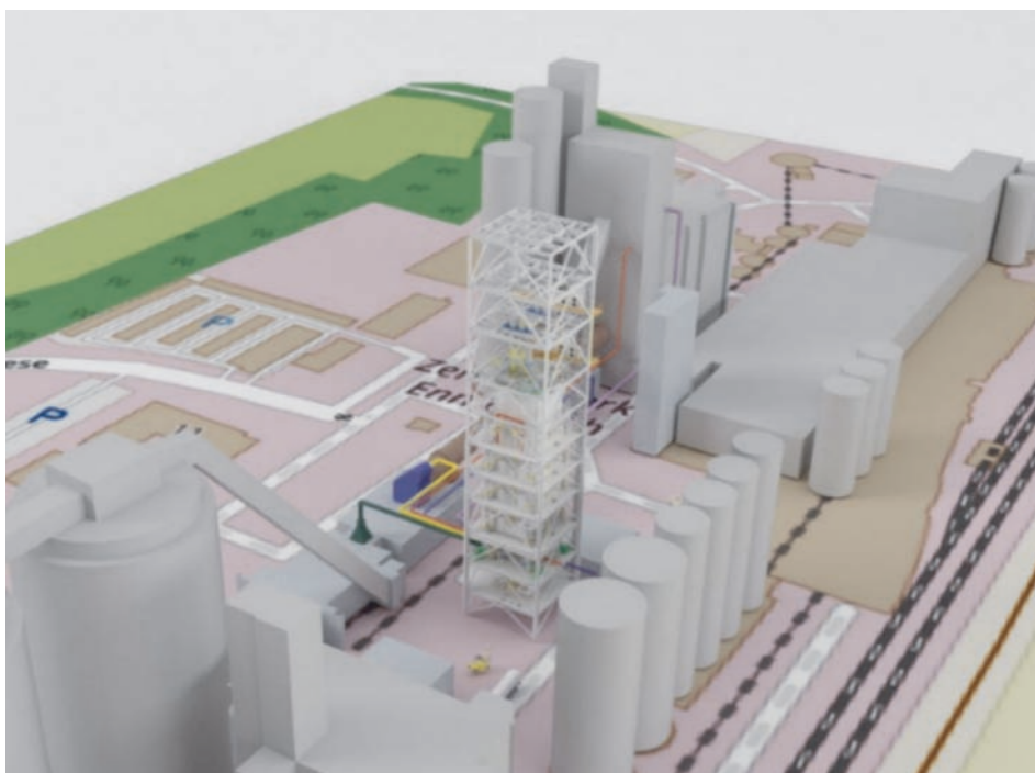
Leilac-2 module located at Heidelberg Materials' Ennigerloh cement plant
